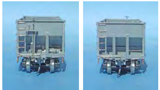
"B" (brakewheel) end detail.(L)"A" end detail.(R)
