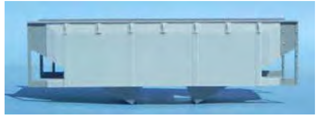
Sides attached, centered on the USRA hopper carbody.
