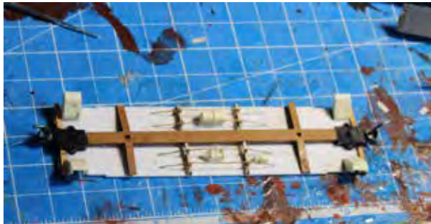
The floor assembly is complete with all the castings from Tichy and AMB installed.
