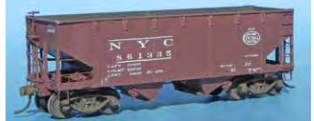
Painted un-weathered model, left side; lettering is from RCW's decal sheet, often requiring modification.
