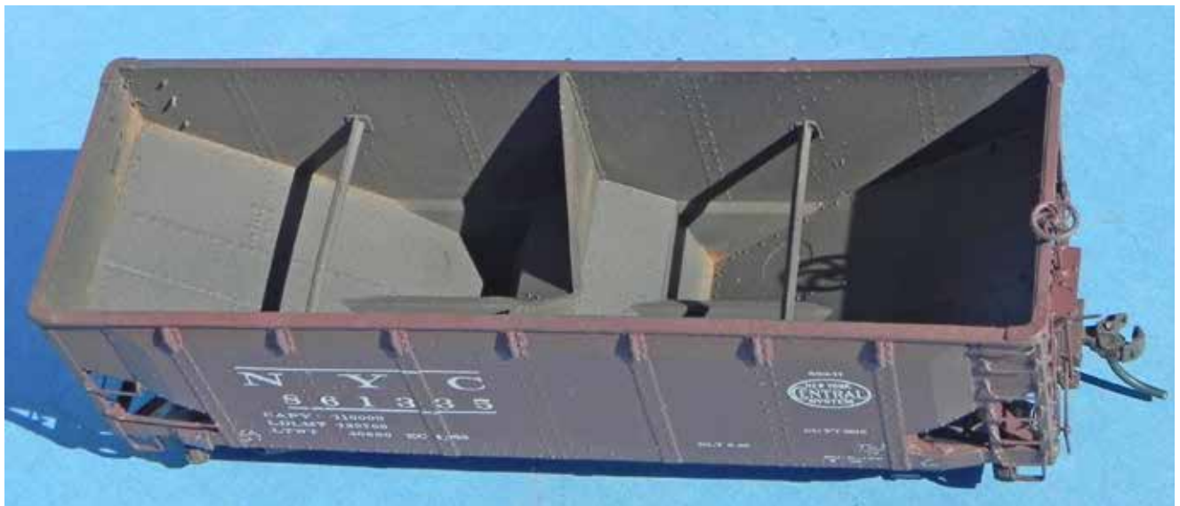
The interior was painted Grimy Black and weathered with a dilute grungy rust overspray; rust at the seams was highlighted with dark rust weathering chalks.
