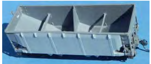
Interior bracing consists of triangular gussets and lateral braces; note small toe-strip on the endsheet interior.
