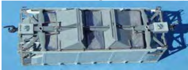
The NYCS elevation was also helpful in placing underbody brake levers and trainline piping.
