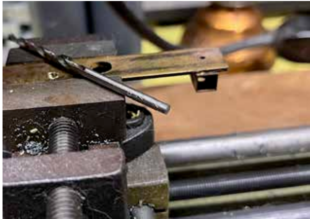
The hole in the plate has been cleaned up so there are no burrs on the plate.
