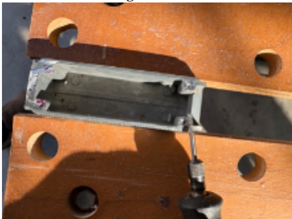
Tom finished the edges with a small sanding bit in his Dremel.
