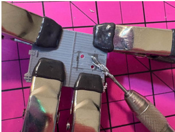
Tom first drilled holes in the structure to enable the cutting out of the door opening.
