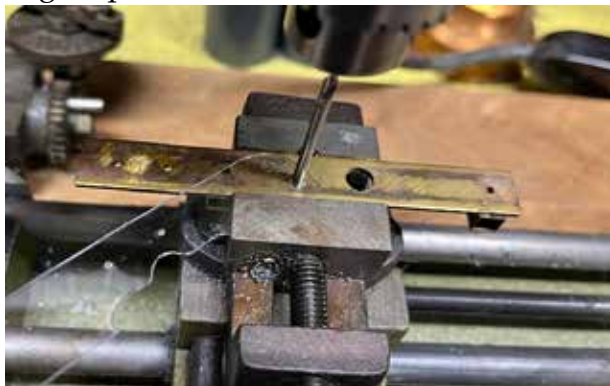
Using the shank end of the drill bit Brian punches out several lens from acetate for his headlights.
