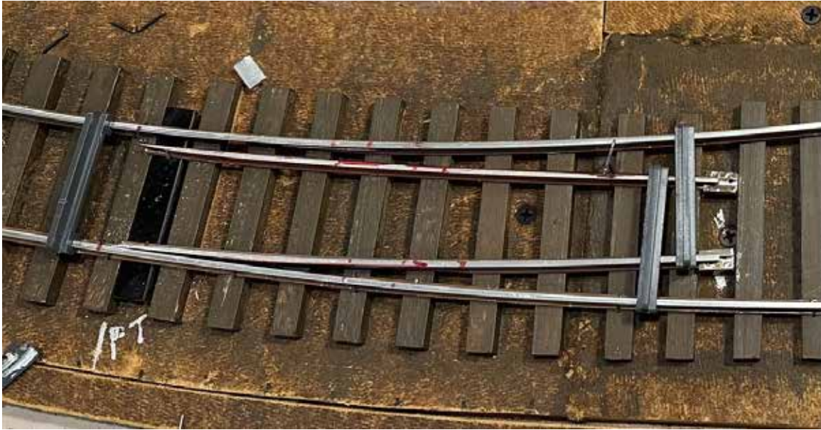
Switch rails fastened to switch rod.
