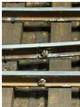
Placement of filister head screws.
