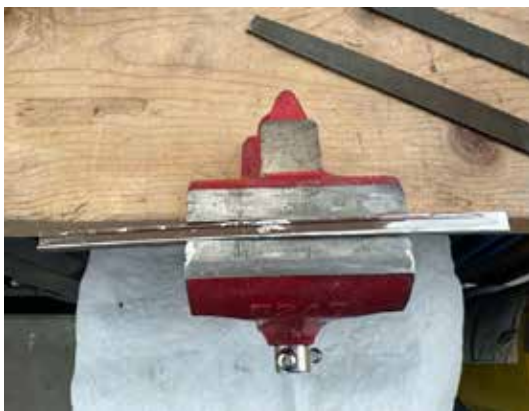
Switch rail in vise during filing the point.
