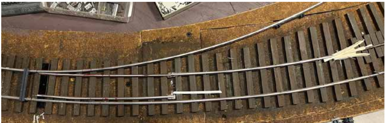
Completed section of turnout without loose parts.
