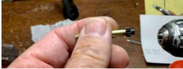
Steve is putting the newly collared shaft in the drill to place the collar in the other end.
