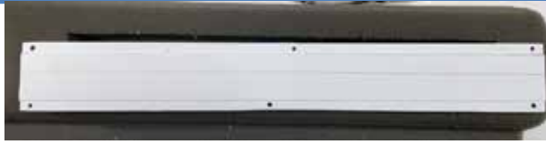
Reinforcement plates glued to the truck bolster.
