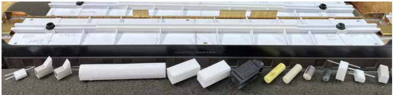
This photo again shows the plastic parts assembled next to the car floor. The fine styrene square used to add hinges and handles to the access doors can be seen before the excess was removed with a sprue trimmer.
