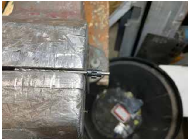
Here is a view of the drill holding the gear. The drill is large enough to act as an axle to allow the gear to spin freely while in the drill chuck.
