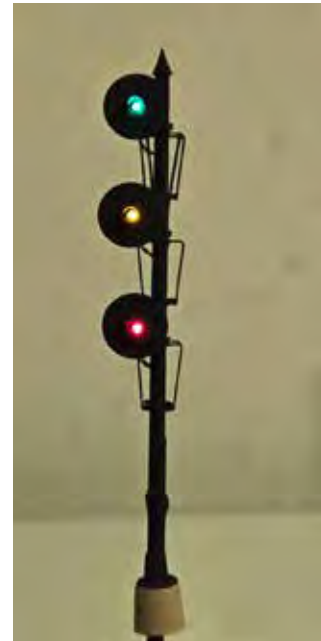
Interlocking signal displaying Rule 281A, green/yellow/red, Advance Approach Medium.
