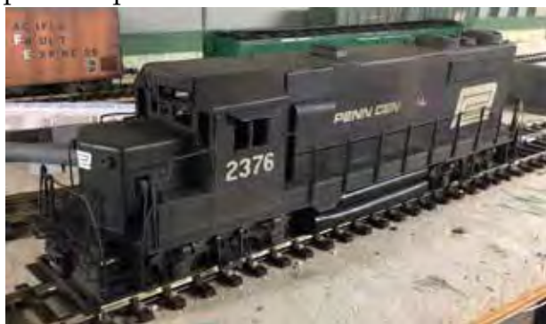
Almost finished is this Central Locomotive Works GP35 kit built without dynamics, its heritage as DRS-14 will be pretty obvious once a few more details are added, like the bell mounted atop the side of the long hood.
