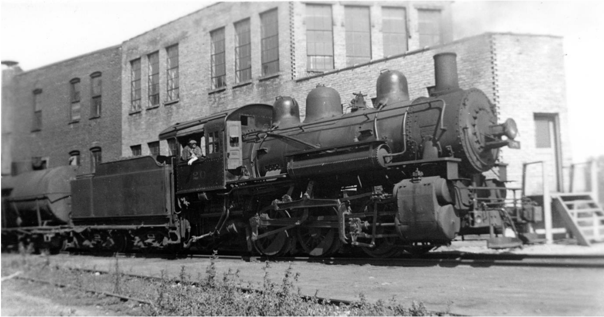
Chicago, Kalamazoo & Saginaw #20 is seen switching in Kalamazoo. A class B-10n 0-6-0, originally MCRR 8779 a Alco product from 1912, it was assigned to the CK&S in 1929, it was retired in 1945. NYCSHS PC528131
